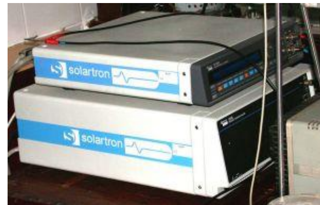
Solartron electrochemical interface+FRA
