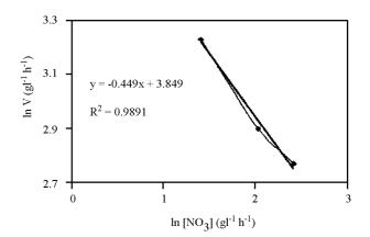
Fig. 6. Denitrifying velocity as function of different initial concentration of ion nitrate
