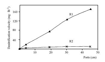
Fig. 5. Denitrifying velocity (12 h HRT) at different ports of R1 and R2
