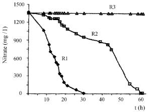
Fig. 2. Comparative kinetic of denitrifying reaction in three column reactors: (R1) packed with *Opuntia imbricate* and consortium; (R2) Consortium without support; (R3) Reactor packed with Opuntia imbricata only
