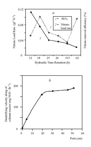
Fig. 3. *a* - Nitrate load rate and removal efficiency of nitrate as function of HRT; *b* - Denitrifying velocity as function of column height at 31.5 h of hydraulic time retention for R1
