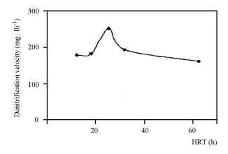
Fig. 4. Effect of hydraulic time residence on denitrifying velocity in the reactor 1
