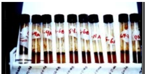
Fig. 1. Test tubes with mineral media containing 3% v/v petroleum applied in Assay for selection of strains. Compare the FIRST TUBE (Control) with the other tubes inoculated with the bacterial strains. Solubility of petroleum in water can be observed in tubes inoculated with bacterial strains
