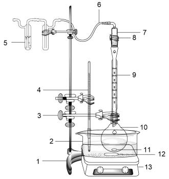
**Figure 1**: 1 = Laboratory stand, 2 = water bath, 3 = clamp holder with clamp, 4 = thermometer, 5 = gas bubbler, 6 = tubing, 7 = hose adapter with inner ground glass joint, 8 = joint clip, 9 = Vigreux column, 10 = round-bottom flask, 11 and 12 = magnetic stir bar, 13 = magnetic stirrer with hotplate
