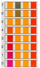
**Figure 3**: Color scale for pH determination by visual comparison with the reaction zones on the indicator strips. All four reaction zones on the pH paper strip have to match the color scale at the given pH value. The pH values are the numbers indicated on the left. You may ask your lab assistant to see the commercial product with the color scale printed on it.
